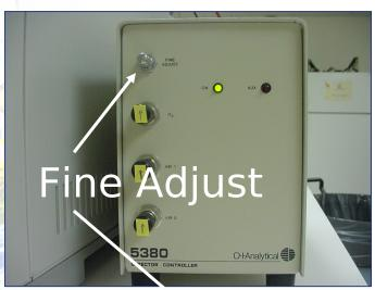
Open the fine adjust needle valve 3 turns (anti-clockwise)
