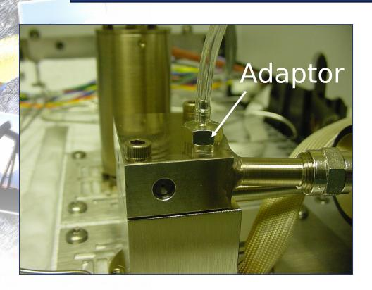
Use the flow measurement adaptor to attach your flow meter
