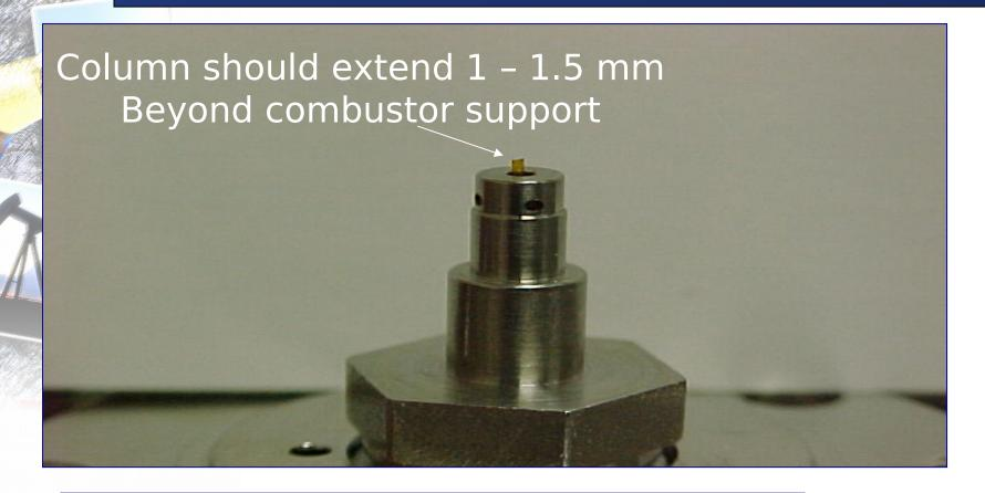
The column can also be installed without the column positioning tool.
