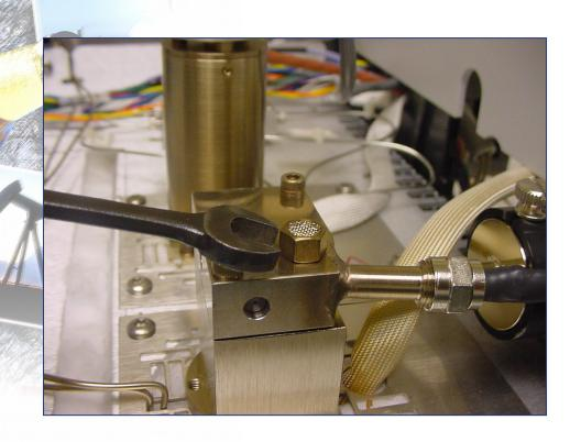
Remove the flow adaptor and reinstall the flame arrestor
