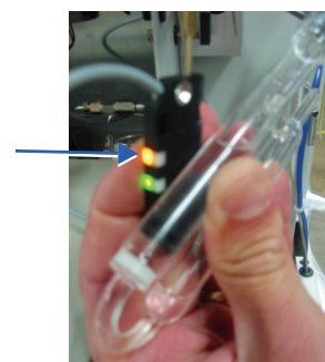
Figure 10.6. Liquid in the sparge vessel actuates the sensor
