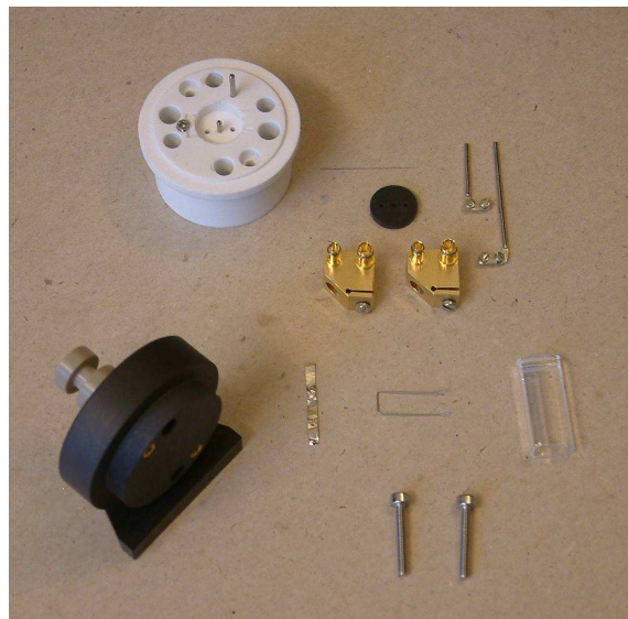
Insert the Pt-flags in the holes in the new septum before mounting it on the probe. Reassemble the probe.
