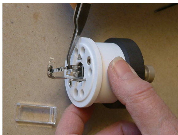
Remove the filament.
