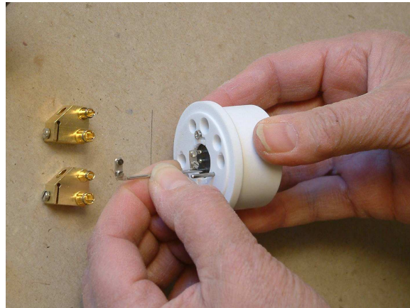
Remove the Pt-flags. Be careful not to damage the flags.
