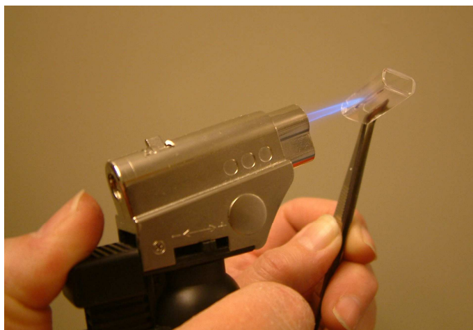
Figure 4-12. Cleaning the glass cell with a micro torch.
