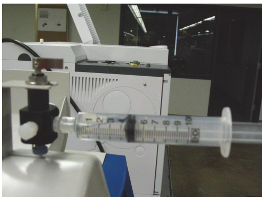
Figure 6.36. Removing the Methanol from the Sparge Vessel
