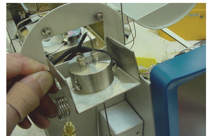
Figure 8.6. Installing the sparge mount bracket
