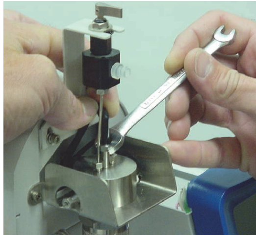
Figure 8.9. Tightening the Foam Buster heater/thermocouple nut
