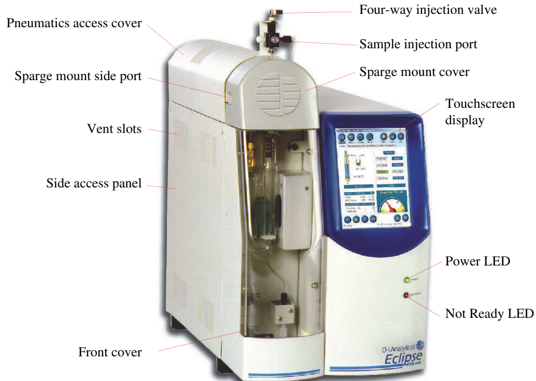
Figure 2.1. Eclipse front exterior components
