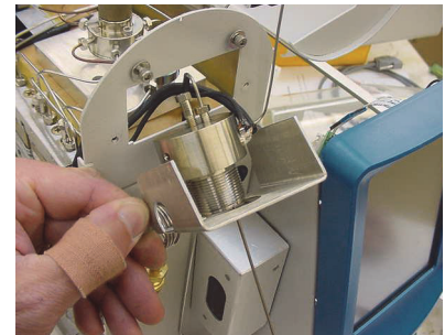
Figure 8.3. Removing the sparge mount bracket
